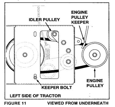
**INSTALLING THE CLUTCH/IDLER ASSEMBLY ON TRACTORS WITH ELECTRIC ATTACHMENT CLUTCHES** (Use these instructions if your tractor has a push/pull switch on the dash panel for starting and stopping the mower deck.)
